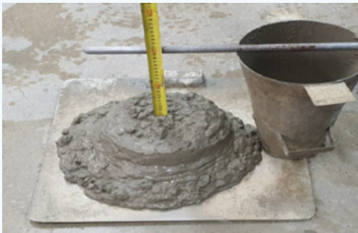
Baseline Slump Shape of Ordinary Portland Cement
